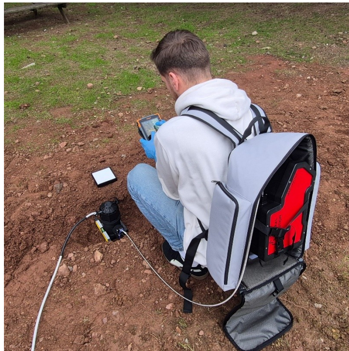
Figure 15. Field measurements with the spectrometer-based portable transfer standard.
