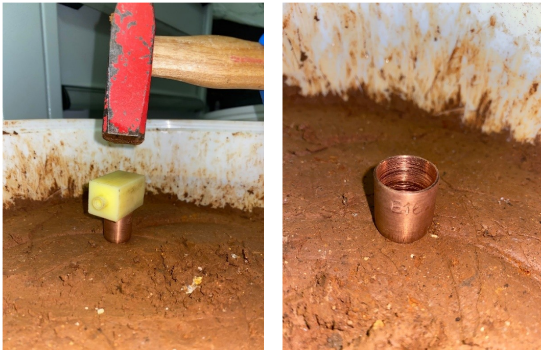
Figure 28. Left: Bulk soil sampling. Right: Ring E16 used to determine the bulk density of the soils used for testing sensor-to-sensor variability.
