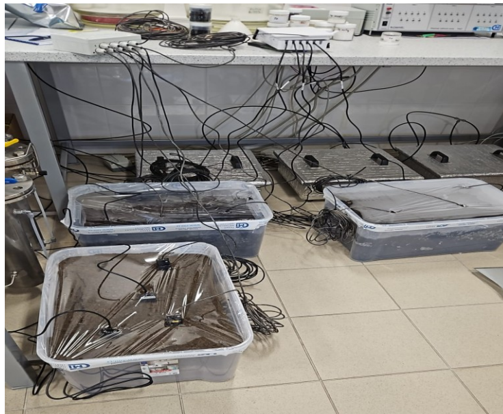
Figure 29. The setup for SMT100 sensors testing – three different soil types.
