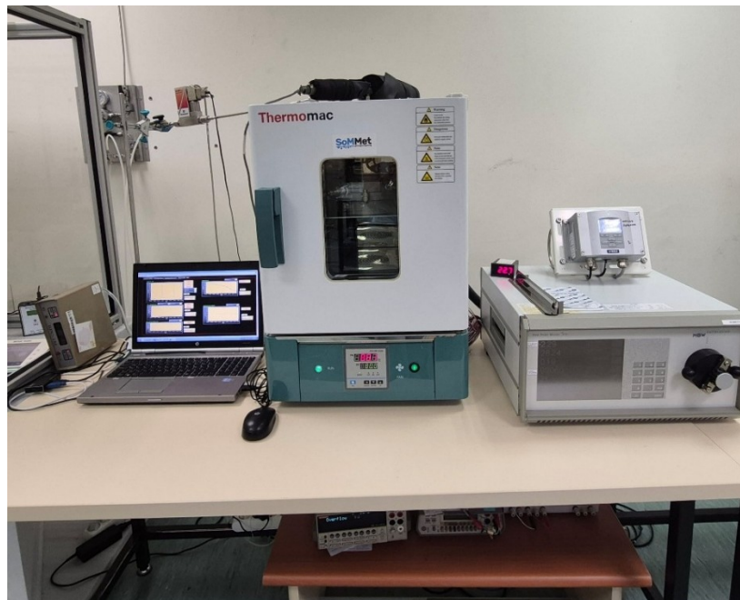
Figure 2. Primary-level Evolved Water Vapour System (EWS) developed by TUBITAK.
