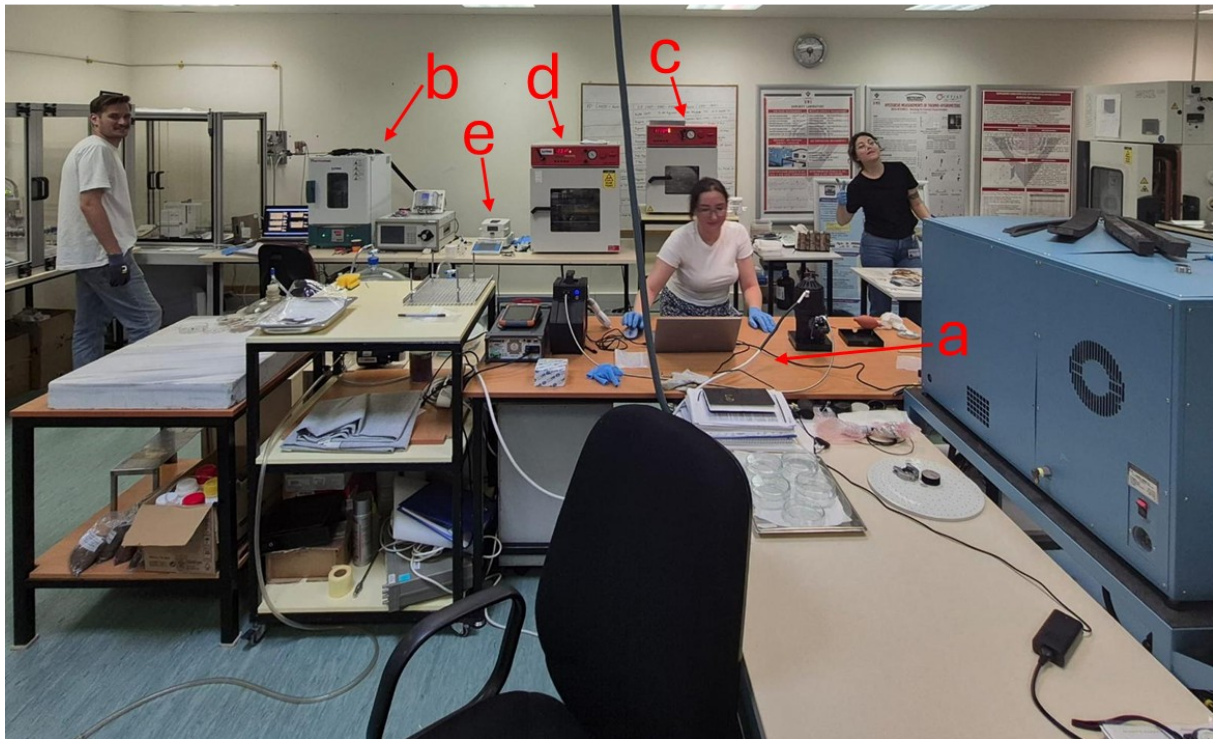
Figure 14. Laboratory setup for simultaneous measurements of soil samples using: (a) spectroscopic system, (b) primary-level soil water content system, (c) LoD system, (d) vacuum-capable LoD system, and (e) laboratory moisture analyser.
