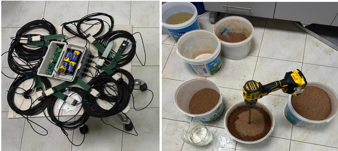
Figure 22. Left: SMT100 sensors. Right: Performing the soil wetting process.
