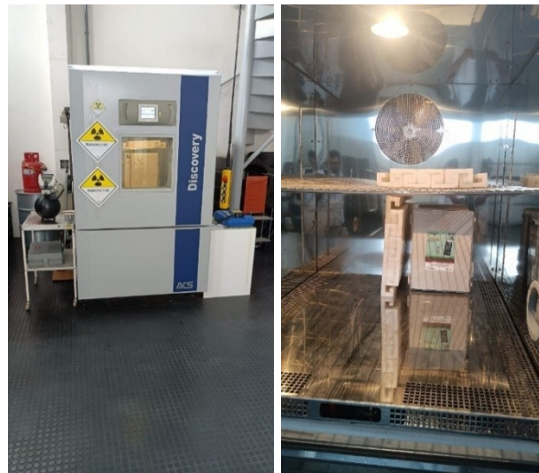
Figure 25. CMI climate chamber with an internal volume of 1 m 3 (left). Detail of the Finapp 3 device during the test inside the climate chamber (right).
