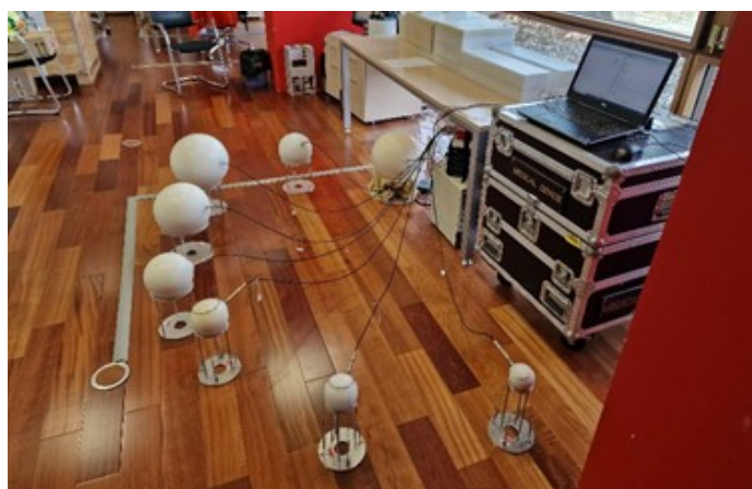
Figure 6. The extended-range Bonner Sphere Spectrometer (BSS) of CIEMAT.
