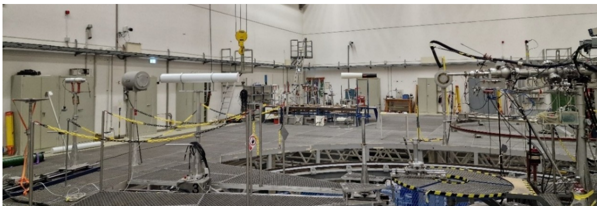
Figure 52. Irradiation of one detector of the CRS-2000/B system aligned with the ion beamline, neutron production target, and the shadow cone.
