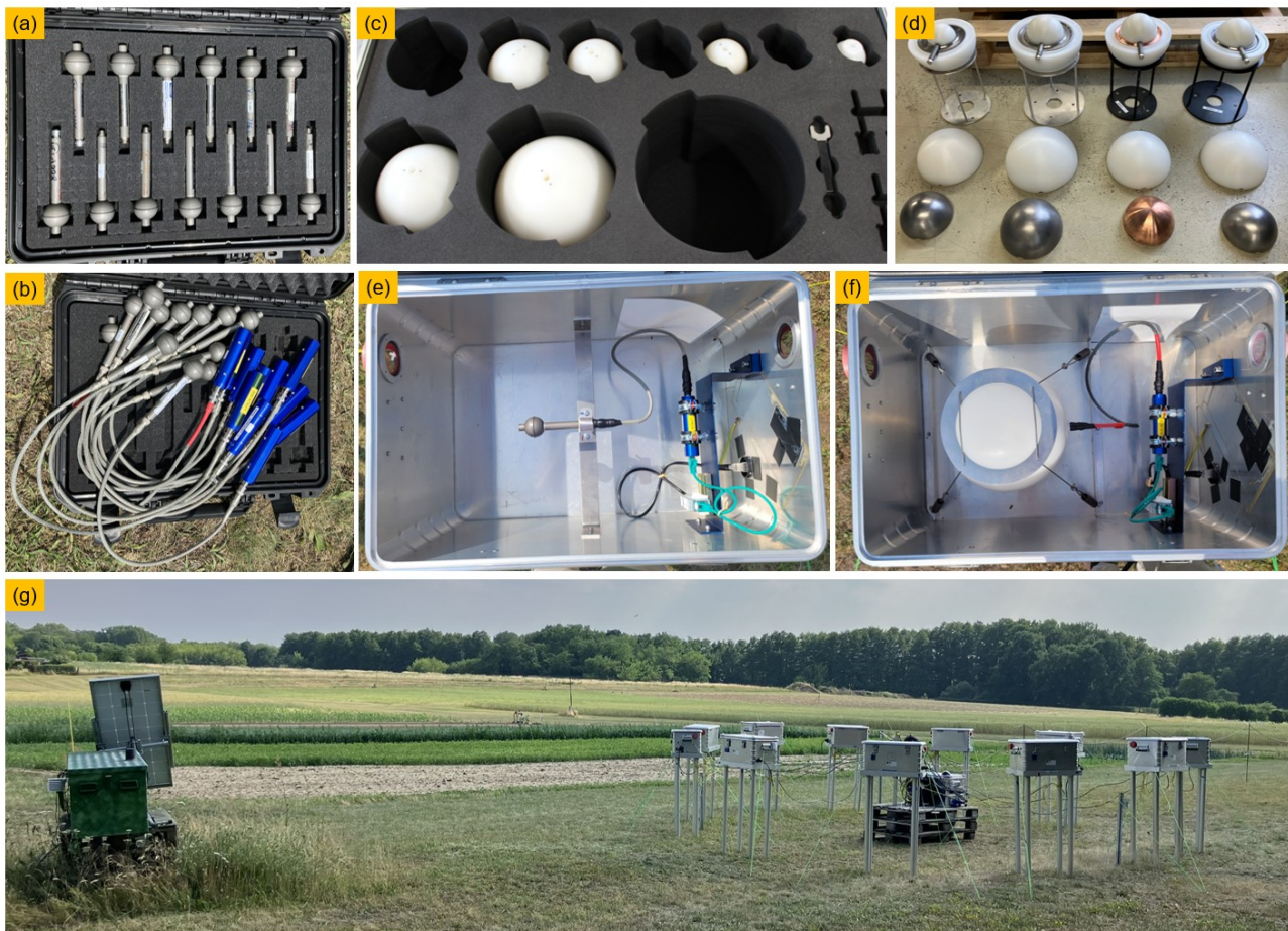
Figure 15. Photographs of the individual components of the PTB Bonner sphere spectrometer NEMUS-UMW for environmental neutron measurements: (a) neutron detectors of type SP9 (Centronic Ltd.); (b) neutron detectors coupled to all-in-one electronic readout modules of type NPM (Neutron Pulse Monitor, Quaesta Instruments); (c) subset of polyethylene neutron-moderating spheres; (d) four “modified” spheres with lead or copper shells for detection of high-energy neutrons; (e) bare SP9 neutron detector and NPM module placed in a weatherproof casing; (f) SP9 detector placed inside an 8-inch sphere and NPM module placed in a weatherproof casing; (g) full setup as deployed at the Marquardt test field site, about 9 metres from CRNS station #31 (visible on the left side of panel (g)).
