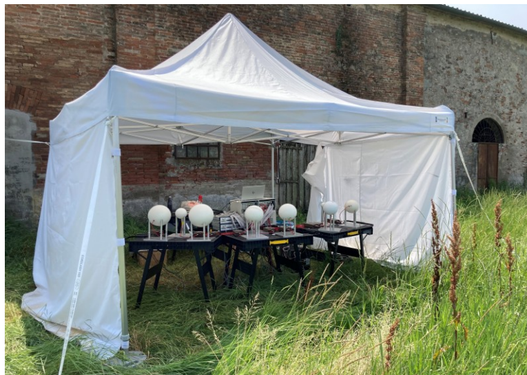
Figure 12. Setup of the HERMEIS ERBSS system of ASNR as deployed for outdoor neutron spectrometric measurements at the Bondeno site.
