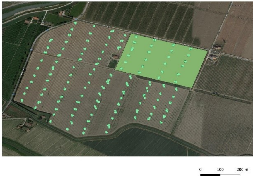
Figure 2. Bondeno agricultural field with TDR surveys. CRNS located on the topright area, marked in green. Positions are marked where surface SWC was measured in field campaigns.
